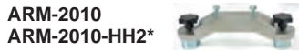
ARM-2010 ARM-2010-HH2* R.E. On/Off Magnet for ARR Rail only Holding power 250 lbs. (113.4 kg) Can be switched on and off for rapid set-up.
