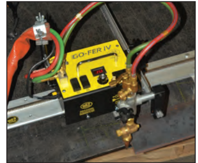
Shown above, oxy-fuel setup of Go-fer IV
