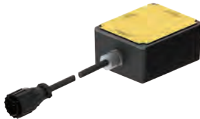
Trigger Adapter Assembly, Push/Pull Uses a 10-pin position connector with pins labeled A-J Uses a 2 position Amphenol with pins labeled A&B for Weld Contact triggering
