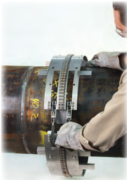
PSR-2000-XX Piper Steel Rail Easily Installed on the workpiece for quick installation and removal
